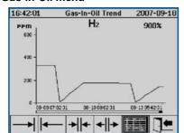
Individual chart diagram for both hydrogen H<sub>2</sub>, carbon monoxide CO and moisture-in-oil (H<sub>2</sub>O in ppm and %)
