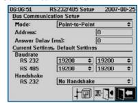
Transmission speed adjustment for the RS 232 / RS 485 connection Different adjustments / settings for the modem communication
